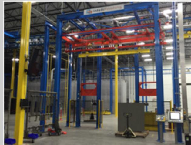
*Lifts are frequently used for IntelliFinishing systems for ergonomic loading and unloading of parts*
